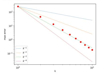
**Observations:** For sufficiently large k ( $k \ge 2$ , perhaps), the slope of the measured errors (red dots) on the log-log plot is at least as steep as -3, as Thm 4.17 guarantees since "n - 1" = 3.
