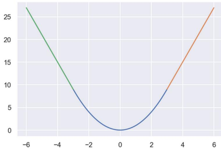
This is continuous, exactly  $y^2$  on  $[-3, 3]$ , but linear outside this interval.
